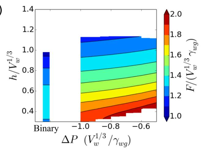
The above demonstrate the effect of varying the pressure difference. Plot (a) shows there is an increase in the breaking separation provided  $\Delta P$  is small enough. Finally plot (b) shows that the smaller the  $\Delta P$  the greater the force.
