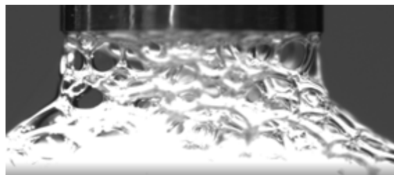
Figure 1: Adhesion tensiometry set-up between foam bubbles to capture the bubble-scale dynamics.
