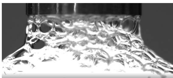
Figure 7: Adhesion tensiometry set-up between foam bubbles to capture the bubble-scale dynamics
